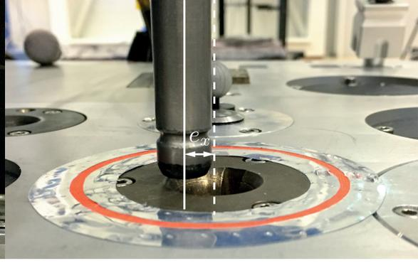
**Figure 3-16:** Example of a translational offset illustrated on the INTERACT task-board.
