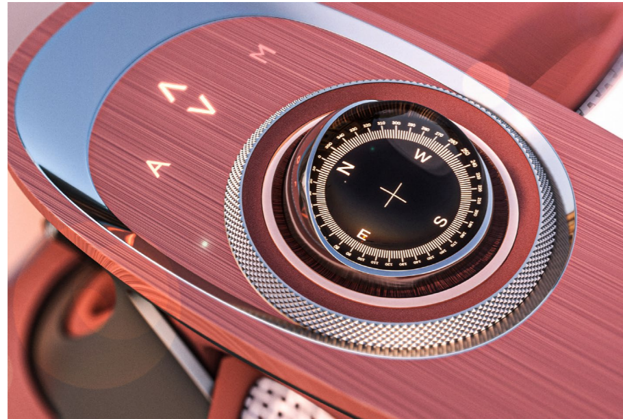
Figure 70. The Navigation Sphere displays in compass mode during autonomous mode, to fully focus on the experience of traveling.
