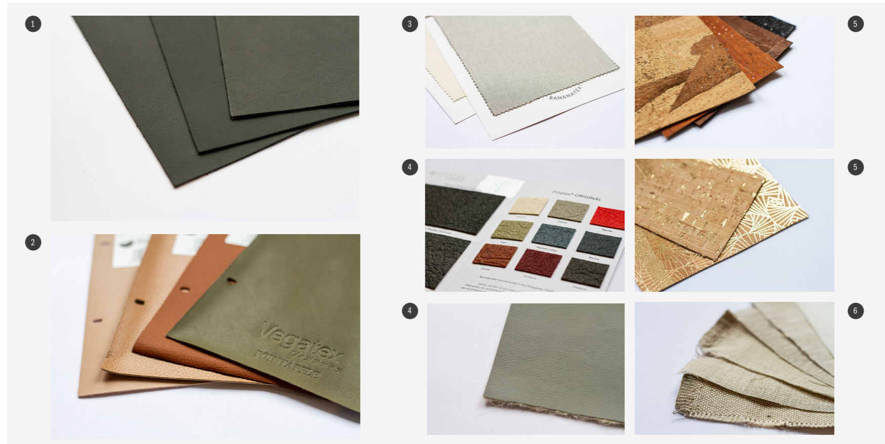
Figure 25. Pictures of the material study. 1) Regular leather; 2) Vegatex Apple Leather; 3) Banatex banana-based leather; 4. Pinatex pineapple-based leather; 5) Cork; 6) Flax.
