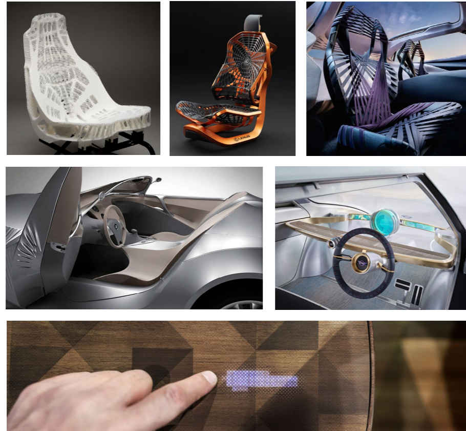
Figure 24. Top: lightweight and tensile seats. Middle: lightweight and simple structures. Bottom: BMW 'Shy Technology', making use of smart surfaces.
