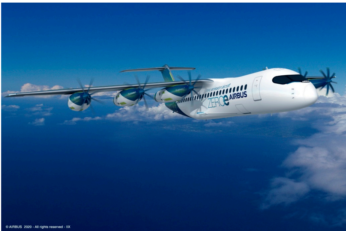
Figure 8-5: One of Airbus ZEROe hydrogen aircraft configuration concepts. In this concept, each propulsion pod contains an \text{LH}_2 tank, fuel cell and electric drivetrain. (Airbus, 2021)
