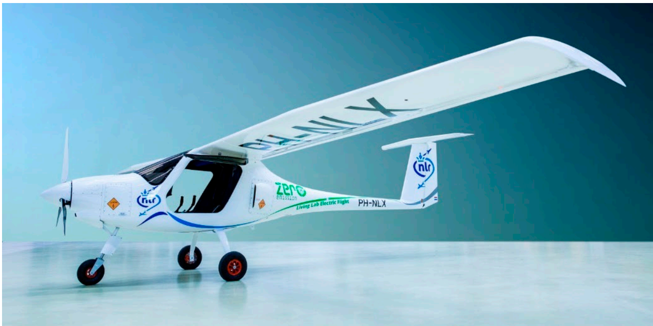
Figure 8-4: Example of certified and commercially available battery-electric aircraft: Pipistrel Velis Electro (NLR research aircraft). Photo © NLR
