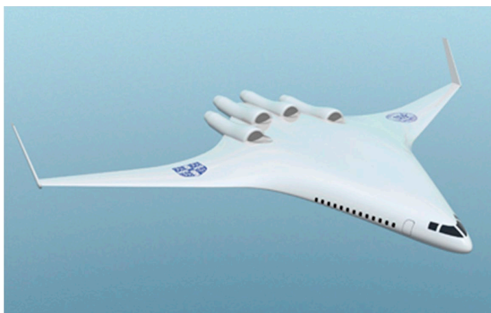
Figure 6-4: Airplane with embedded engines (distorted flow causes much additional noise and is a threat to fan structural integrity expected (Michel, 2011))
