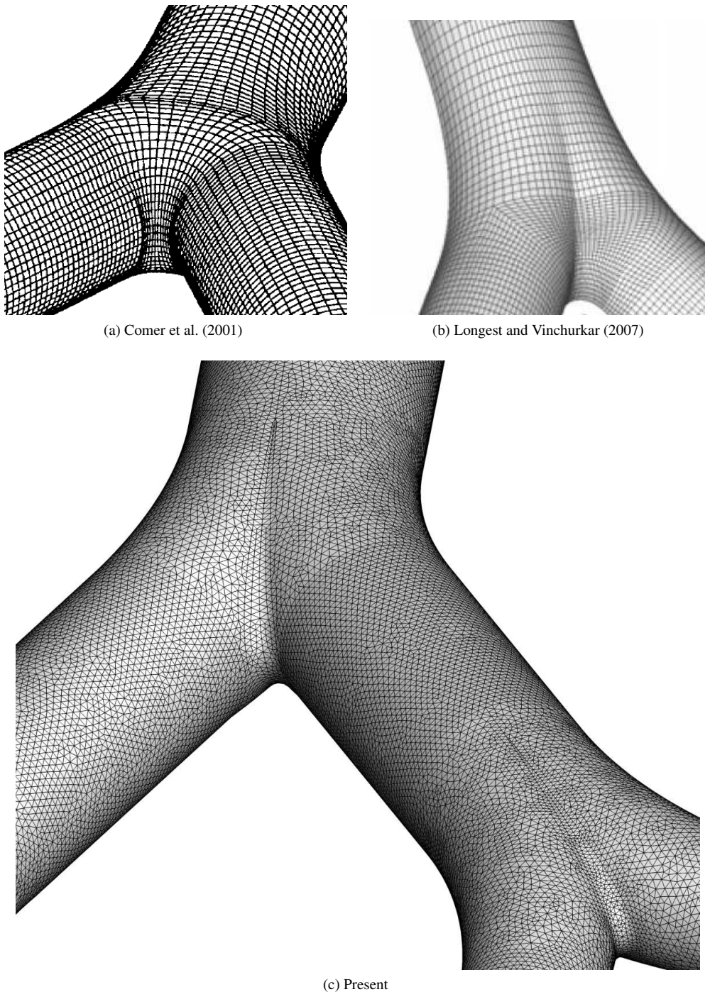
Figure 7.2: (a) Mesh at the bifurcation region in the geometry by Comer et al. (2001). (b) Mesh at the bifurcation region in the geometry by Longest and Vinchurkar (2007). (c) Mesh used in the present study.
