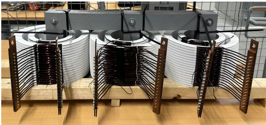
Figure 7.23: Assembled medium-frequency transformer (MFT) with winding modules secured and core clamped in place.
