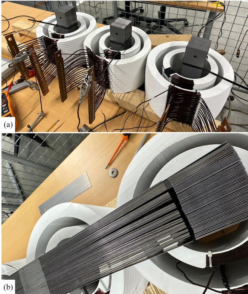
Figure 7.22: Alternative assembly method where the magnetic core is first fully assembled, and: a) the upper yoke is removed to allow winding insertion; (b) after positioning the windings, the upper yoke is reinstalled piece by piece to complete the magnetic path.
