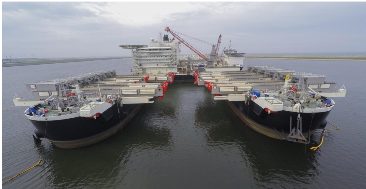
Figure 1.1: The topsides lift system of Pioneering Spirit, with four forklift units on each side
