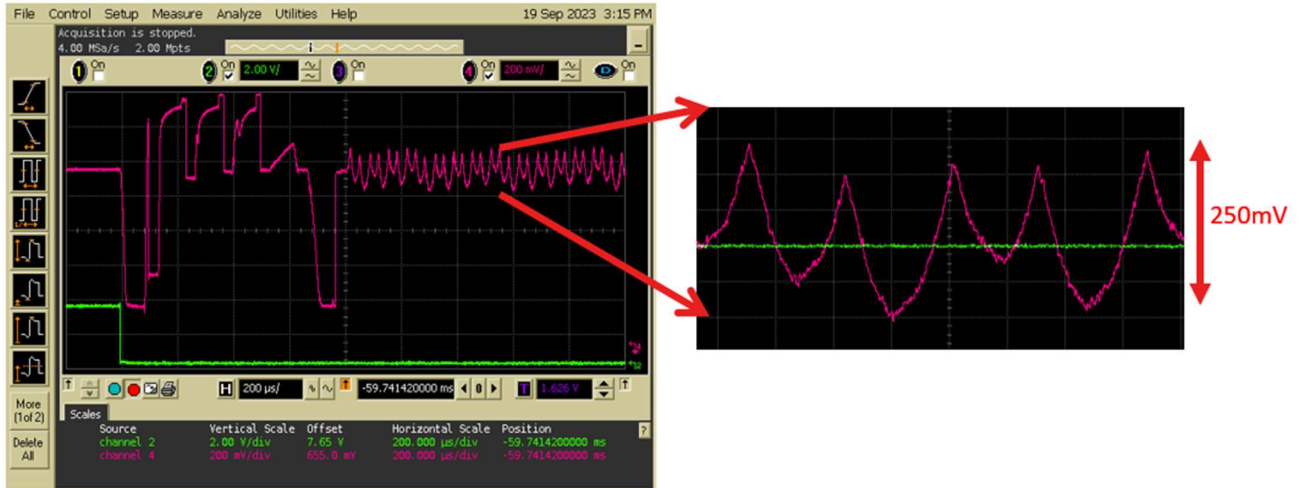
Figure 4.8: PD-DSM's Integrator output after SAR trim and RRL.
