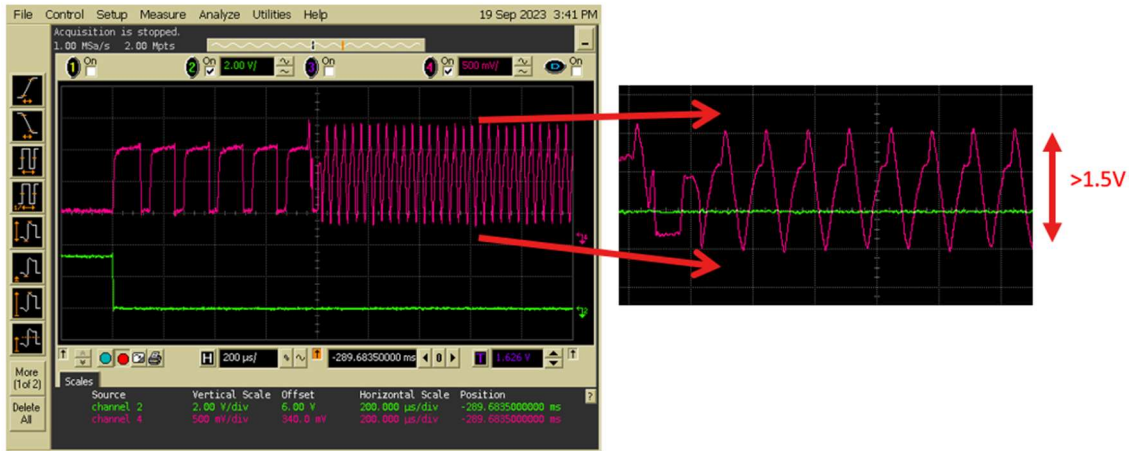
Figure 4.4: PD-DSM's Integrator output w/o SAR trim, w/o RRL.
