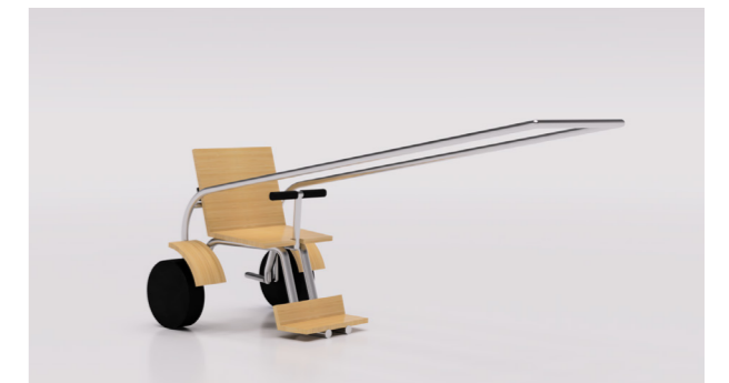
Figure R.3: Double tubes to footrest, single suspension
