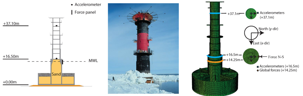
Figure 2. Illustration, picture and finite element model of the Norströmsgrund lighthouse, from Nord et al.
