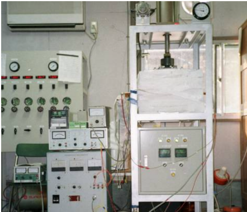
Figure B1: MCFC bench cell setup at Tohoku University. MCFC manufactured by IHI.
