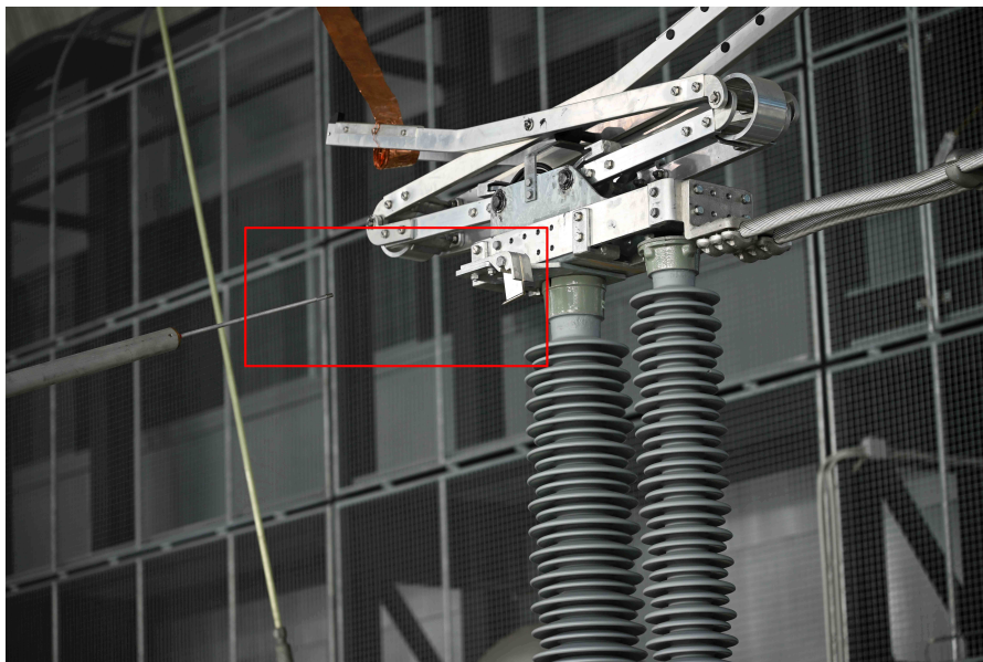
Figure 5.21: Earthing contact - needle gap
