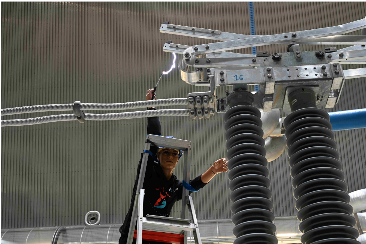
Figure 6.8: Mannequin placed deliberately too close to the busbar disconnector with an applied switching impulse
