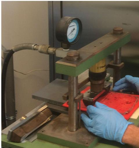
Figure 3.5: The process of die cutting the amnion.
