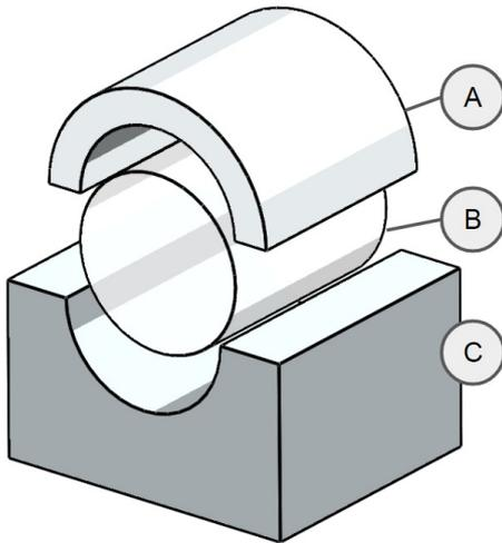
Figure 2.1: The three main conceptual components, from top to bottom: A: artificial abdominal wall, B: artificial abdominal cavity and C: the trestle frame.
