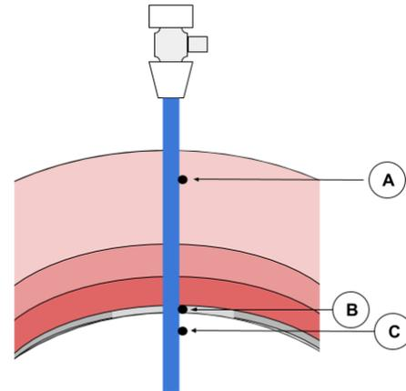
Figure 3.12: Schematic of the locations of the sensors in a cut-section of the abdominal wall. A: Top sensor, B: Reference at amnion location, C: Inner sensor.
