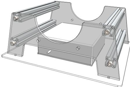
Figure 3.10: Sub-assembly of the trestle frame, including the aurora measurement system.
