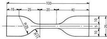
Figure 3.4: Technical drawing of the in ISO 37-1A specified test specimen.
