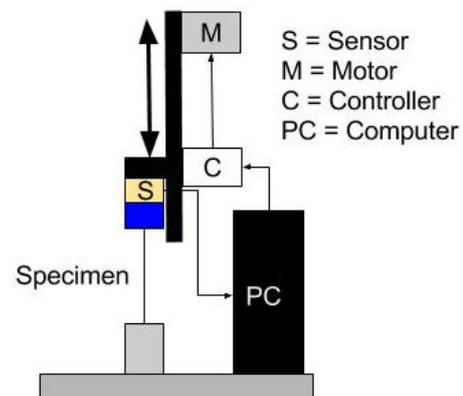
Figure 3.7: Schematic overview of the linear stage used for this experiment.
