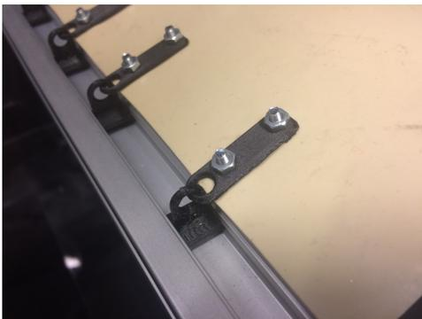
Figure 3.3: 3D printed hinges to move the skin layer and expose the underlying structure.
