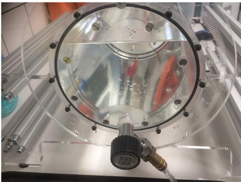
Figure 4.1: A photo of the testing of the model for water tightness.
