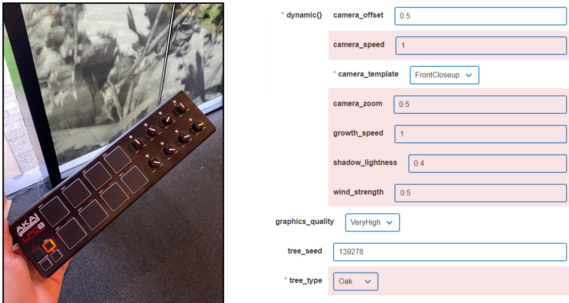
Figure 4.8: Adjustable parameters through the remote controller (left) and through the website access (right).
