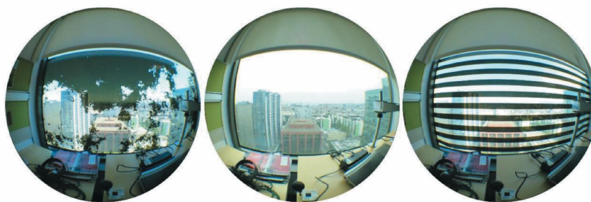
Figure 2.9: Window patterns tested: fractal pattern D = 1.7 (left), clear condition (middle), and striped pattern D = 1 (right) (Abboushi, Elzeyadi, Wymelenberg, et al. 2021).
