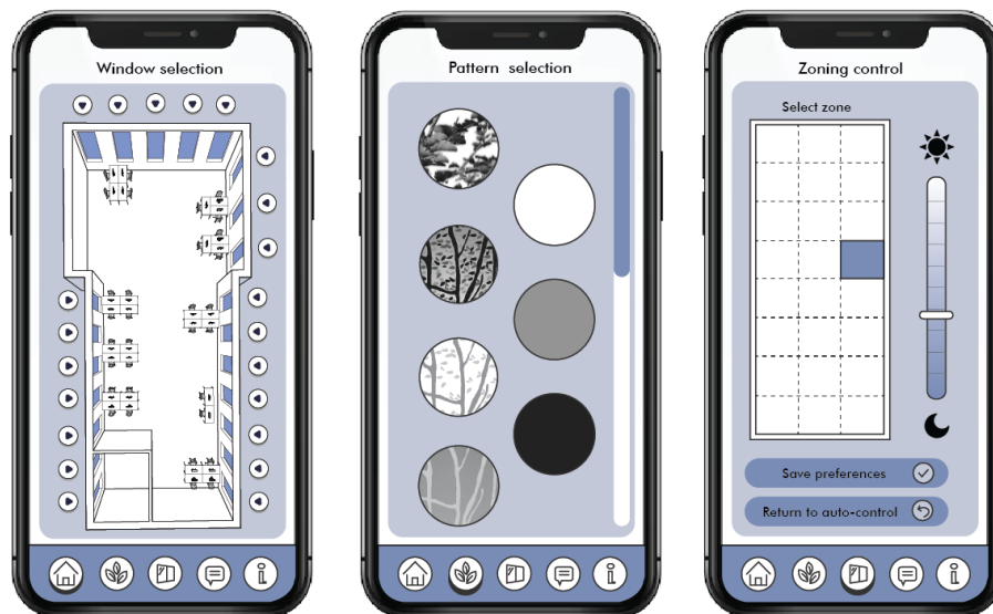
Figure 7.6: Example of interface that could enable personal control of the pattern presence by the user, selection of window of interest for adjustments (left), select pattern for window exposure (middle), adjust transparency through zonal control of the window (right).
