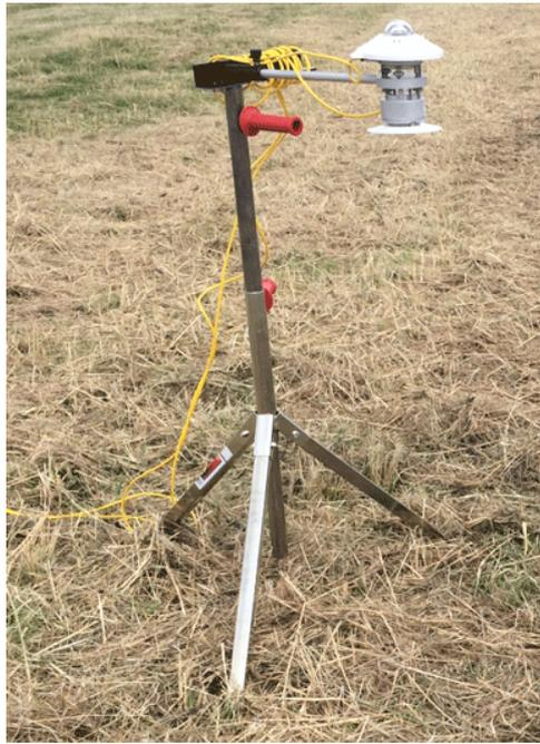
Figure 3.5: The albedometer that was used for the measurements.
