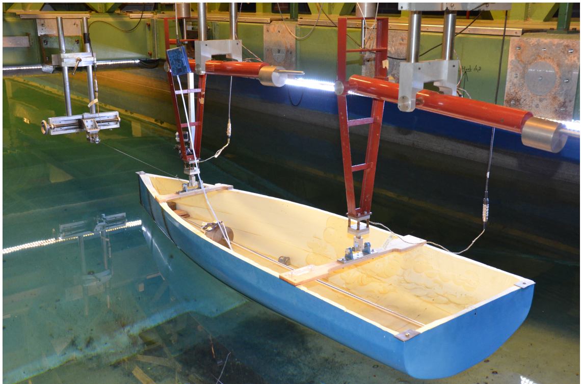
Figure 8.1: A picture of the measurement set-up that was used for the resistance measurements. Figure from Kleijweg [31].
