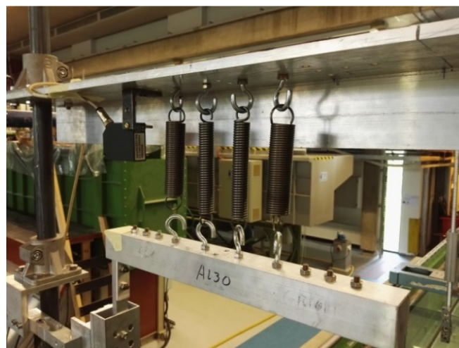
Figure F-8: Picture of spring connection between internal frame and external frame
