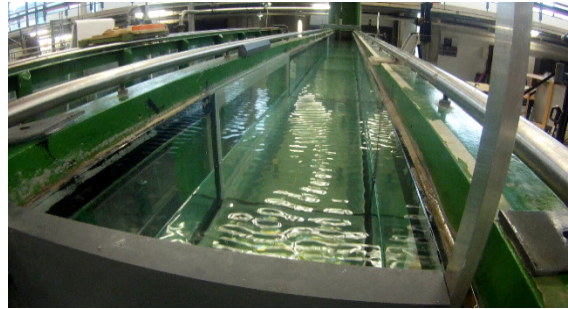
Figure 4-15: (L) Test with clear vibrations visible & (R) Picture of visible small period waves due to vibrations of the valve
