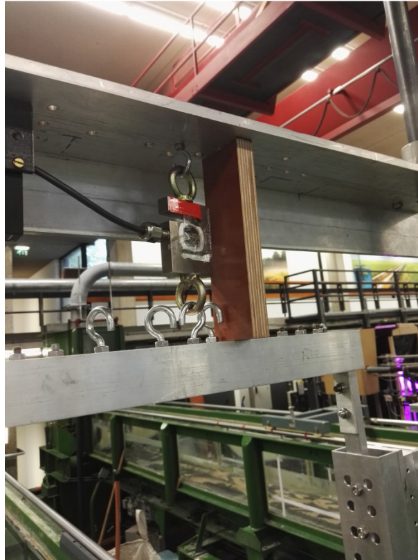
Figure F-9: Extreme stiff vertical suspension
