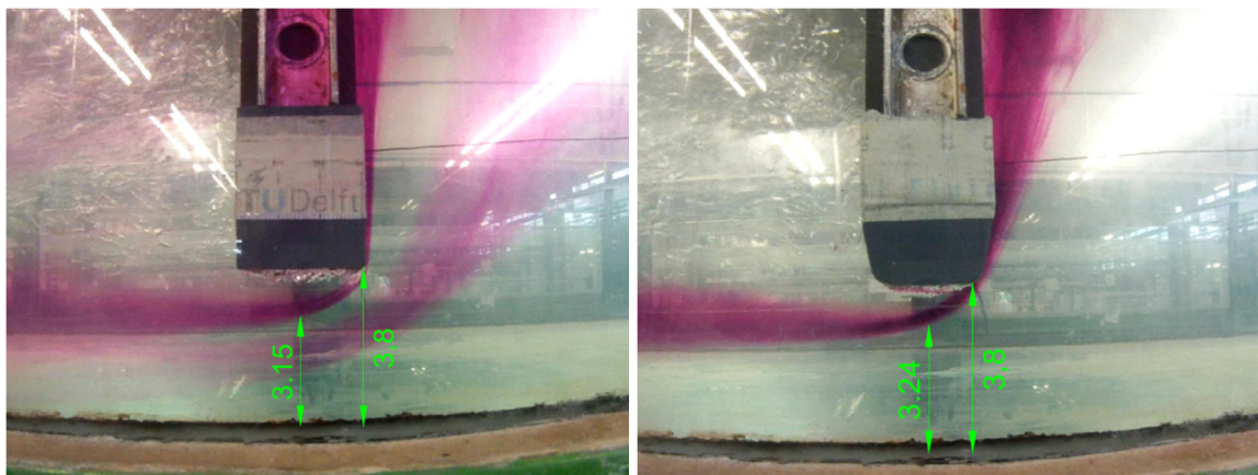
Figure 4-29: Determination of contraction underneath the valve for the rectangular-shaped seal (L) & the chamfered-shaped seal (R)
