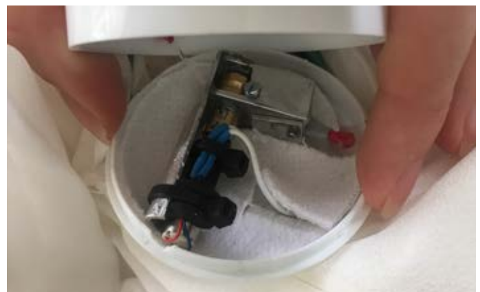
figure 107. DC motor as a friction wheel drive mechanism
