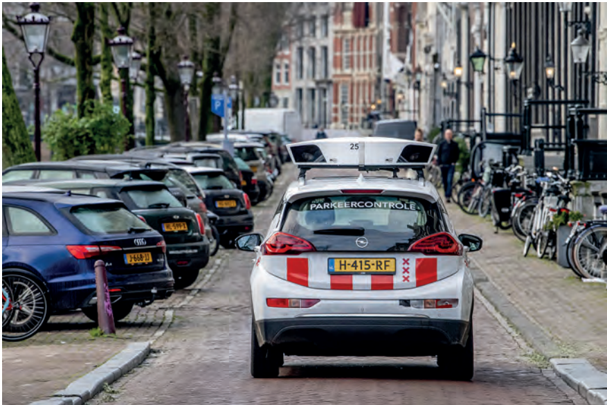
Figure 1.2 A parking monitoring camera car driving through the streets of Amsterdam. (Photo: Robin Utrecht)
