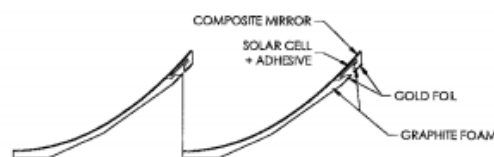
Figure 2.7: Deep Space concentrator element design from the patent [22].
