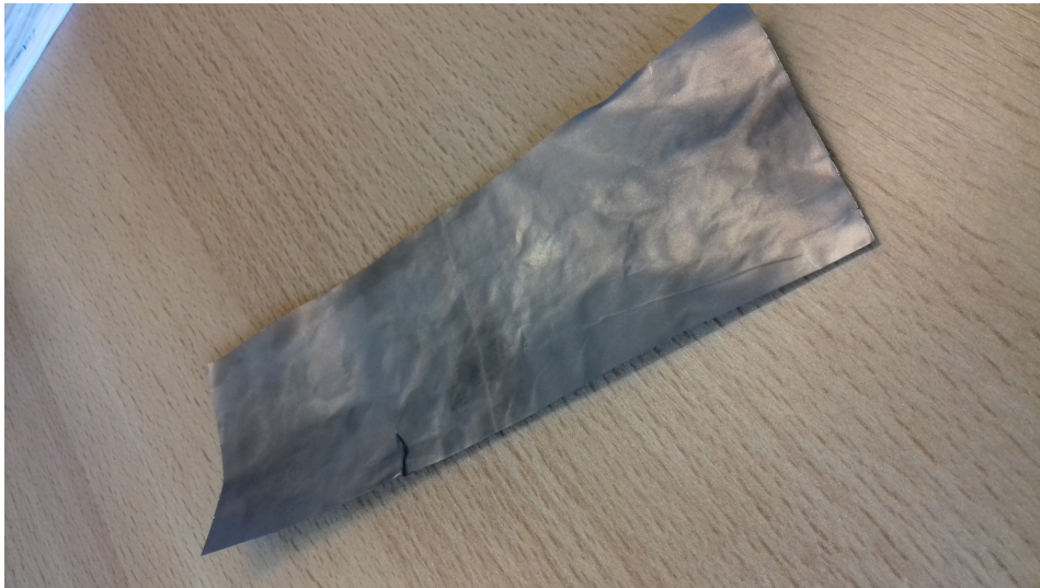
Figure 5.10: Single layer of pyrolytic graphite.
