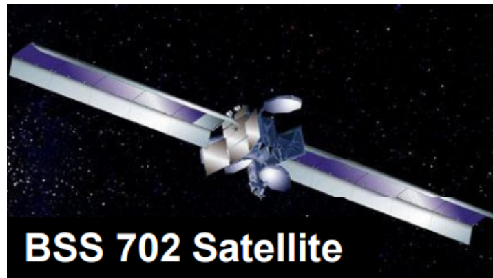
Figure 2.4: Panel edge reflectors used on the Boeing 702 [18].
