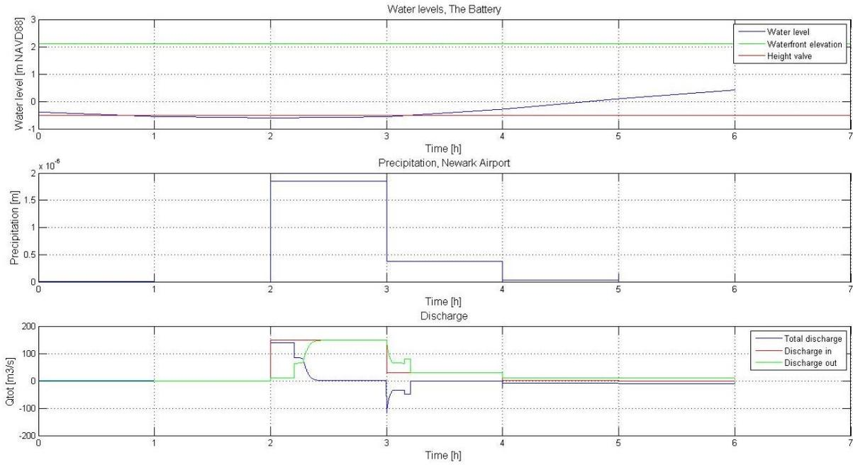
Figure 27 Model results of an extreme rainfall event Hoboken: Water levels (plot 1); Precipitation (plot 2); Inflow and outflow fluxes (plot 3)
