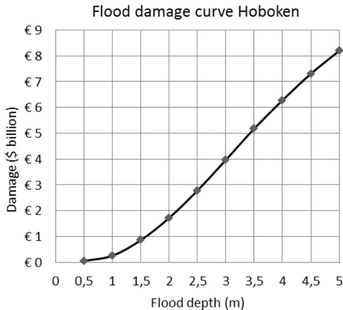
**Figure 44** Damage curve Hoboken
