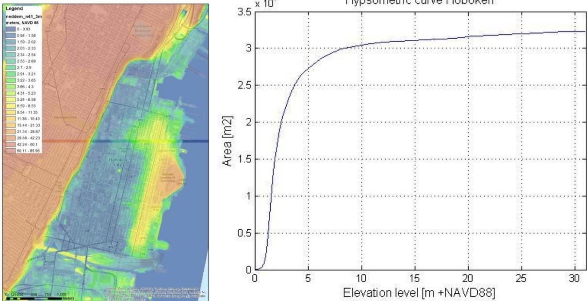
Figure 11 a) Digital Elevation Model Hoboken (left); b) Hypsometric curve Hoboken
