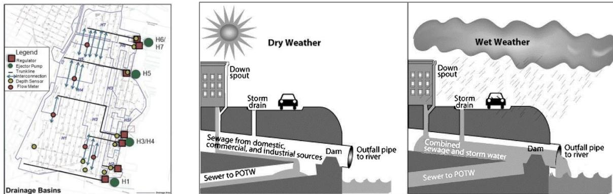
Figure 14 Drainage basins (EmNet, 2011); Combined Sewer Overflow Hoboken (OMA, 2014)
