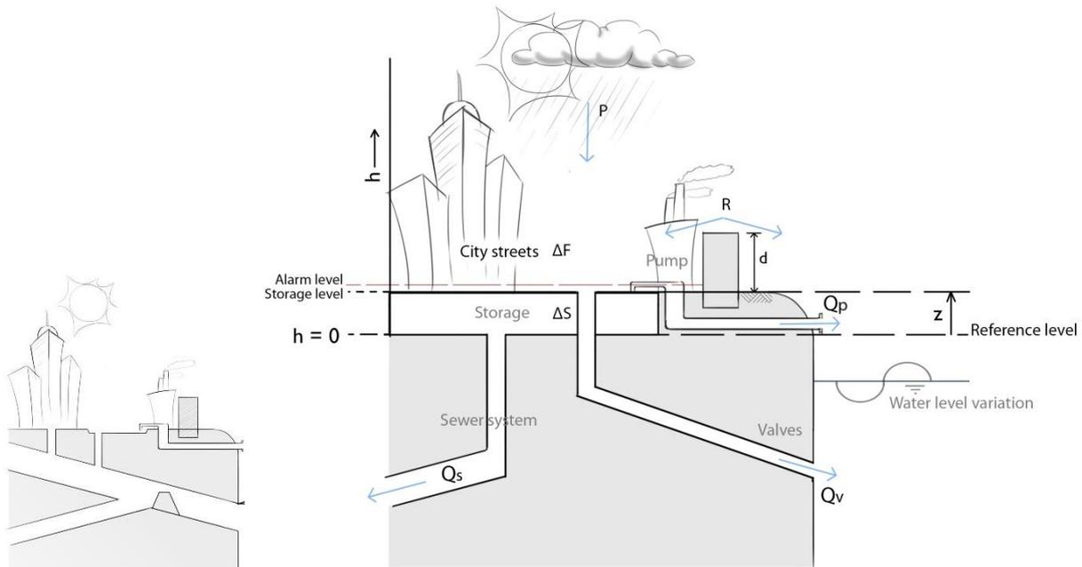
Figure 18 Schematization of a city in the model (left: actual lay-out; right: model lay-out)
