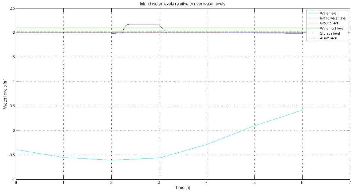
Figure 29 Model results of an extreme rainfall event Hoboken: Outside water level; inland water level; important limit levels
