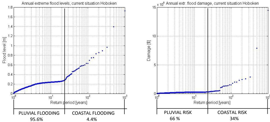
Figure 45 Current situation return periods flood levels and damage in Hoboken
