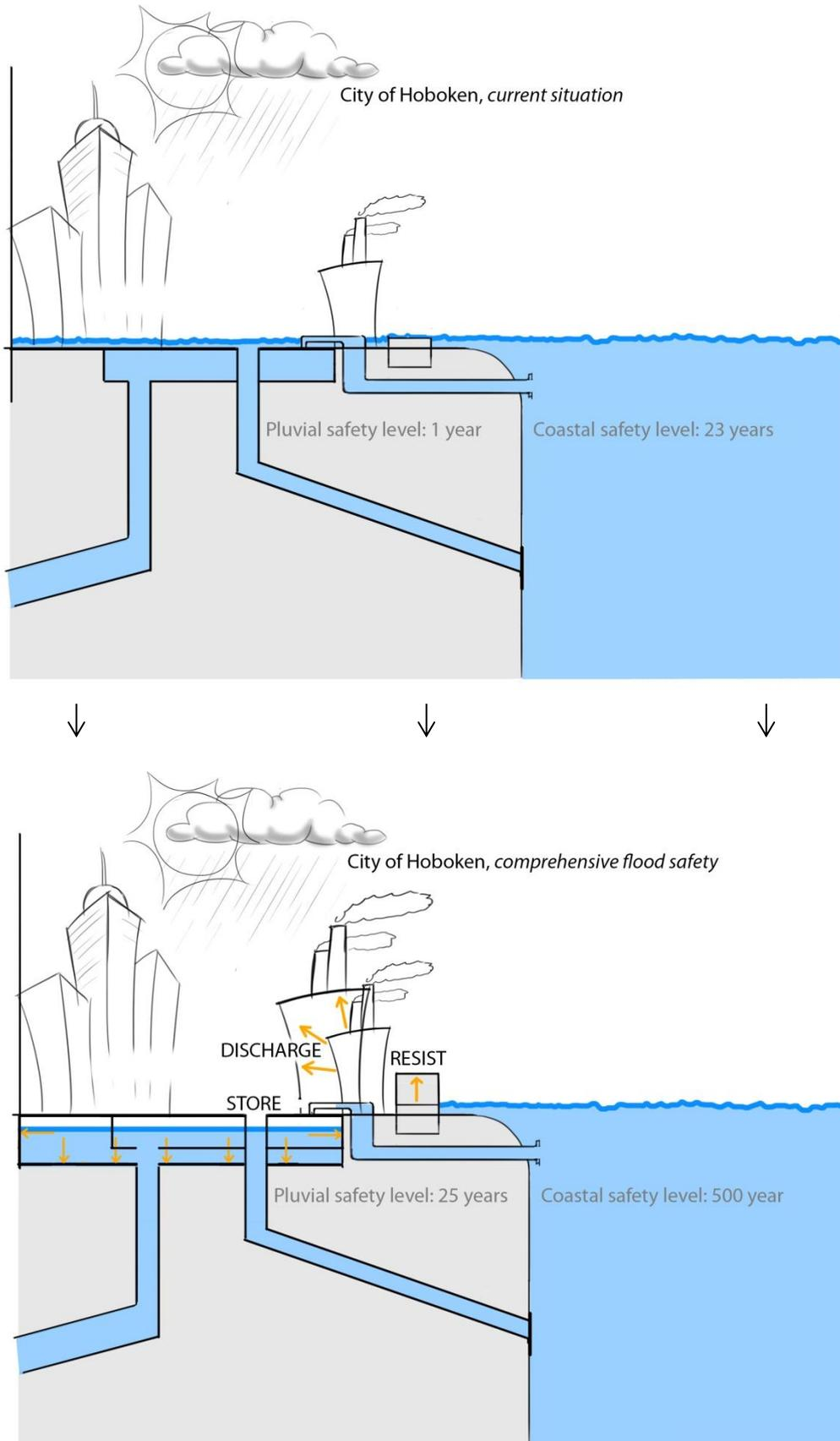
Figure 51 Optimal combination of flood risk reduction measures in Hoboken (before and after)
