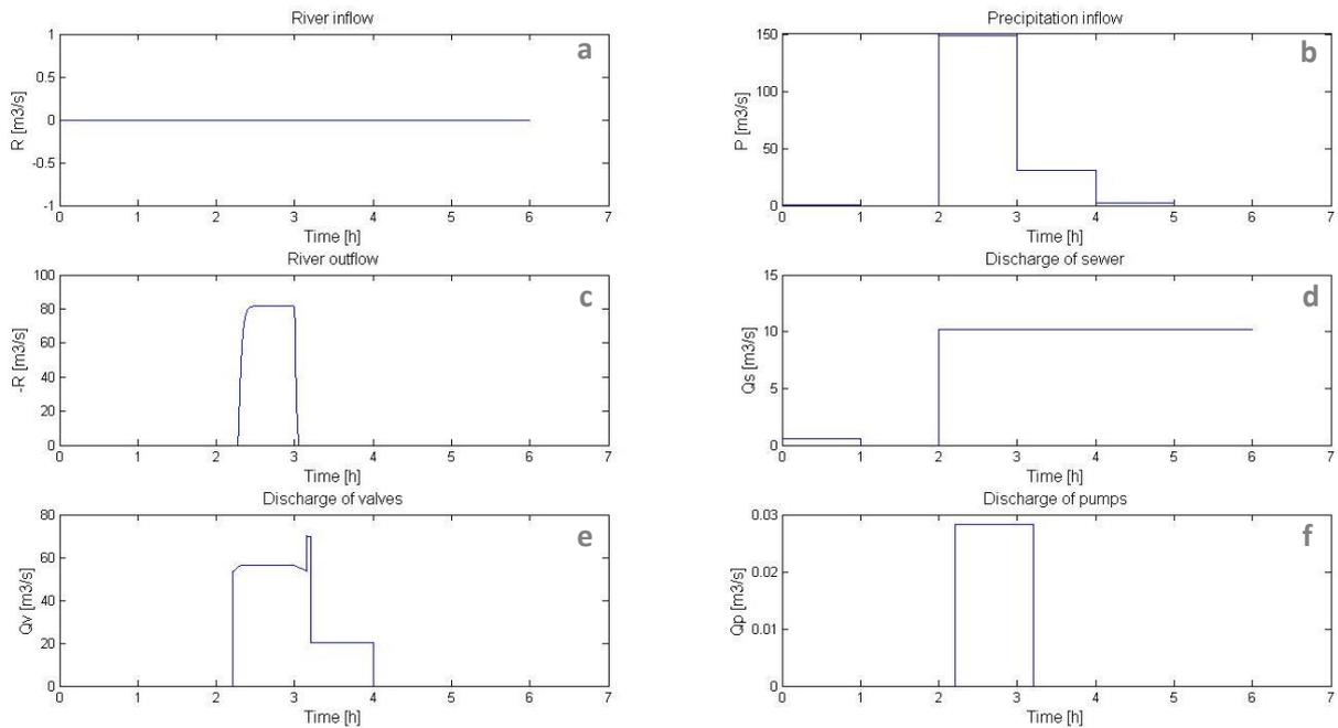
Figure 28 Model results of an extreme rainfall event Hoboken: River inflow (plot a); Precipitation inflow (plot b); River outflow (plot c); Sewer discharge (plot d); Valve discharge (plot e); Pump discharge (plot f)
