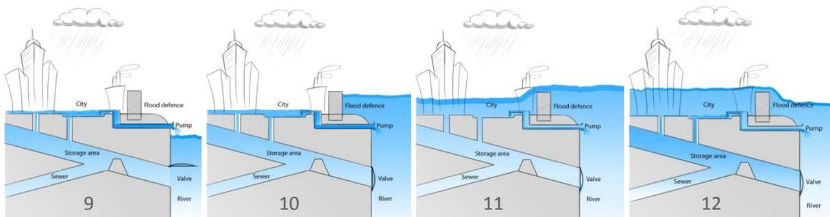
**Figure 20 Humid or extreme weather; pluvial, combined or riverine/coastal flood**
