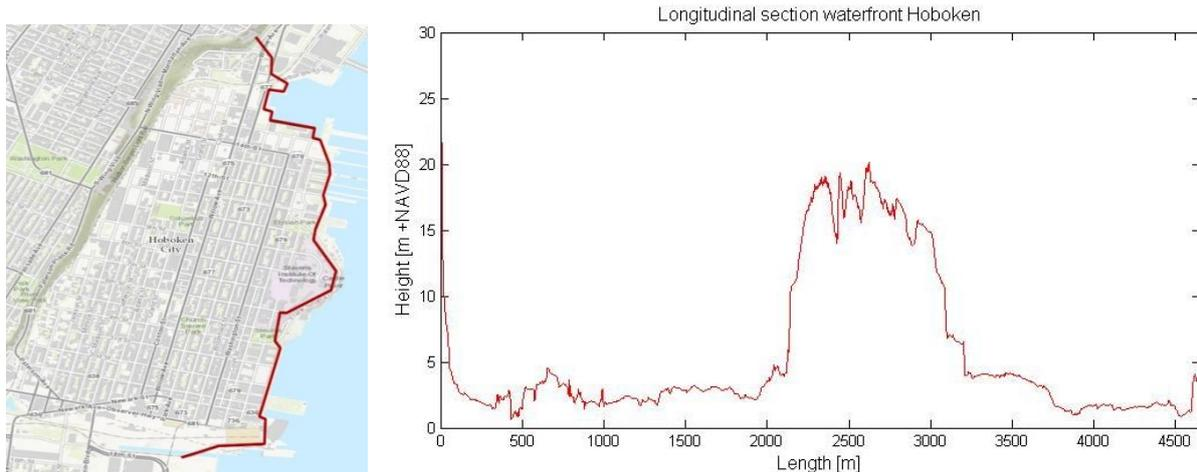
**Figure 12 a) Location longitudinal section waterfront Hoboken (left); b) Longitudinal section waterfront Hoboken from south to north (right)**
