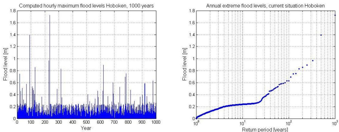
Figure 40 Computed flood levels (left), Right: Computed annual extreme flood levels (Hoboken, 1,000 years)
