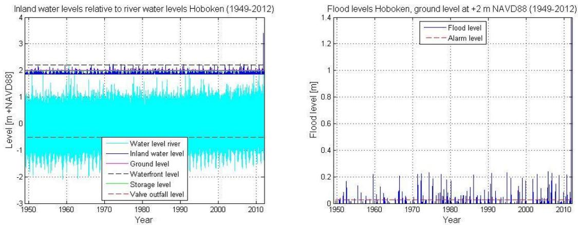
**Figure 33 Hoboken 1948-2012: Inland water levels relative to river levels; flood levels**
