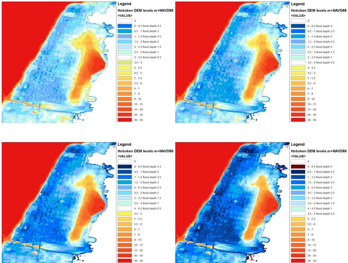
Figure 42 Flood maps Hoboken, varying from 0 to 5 m flood depth (ArgGIS)
