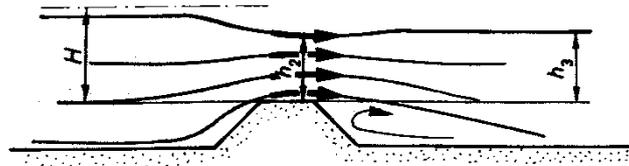
Figure 21 Flow over weir (Nortier, et al., 1994)
