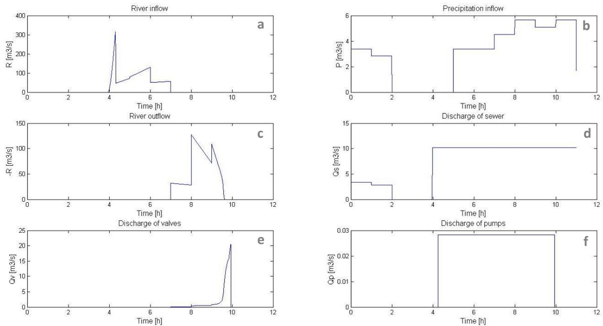
**Figure 25 Model results during overflow (Hurricane Sandy Hoboken): River inflow (plot a); Precipitation inflow (plot b); River outflow (plot c); Sewer discharge (plot d); Valve discharge (plot e); Pump discharge (plot f)**
