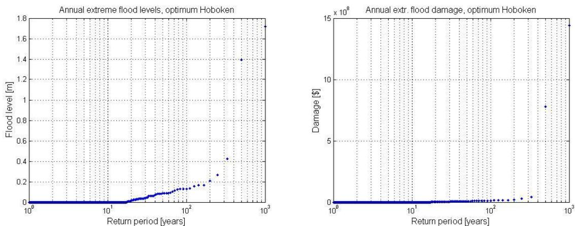
Figure 50 Ranked annual maximum flood and damage levels optimal combination (0.8 m; 5 ha; 92,100 m<sup>3</sup>/h)
