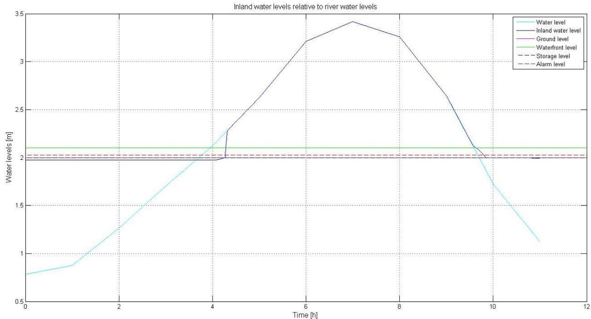
**Figure 26 Model results during overflow (Hurricane Sandy Hoboken): Outside water level; inland water level; important limit levels**
