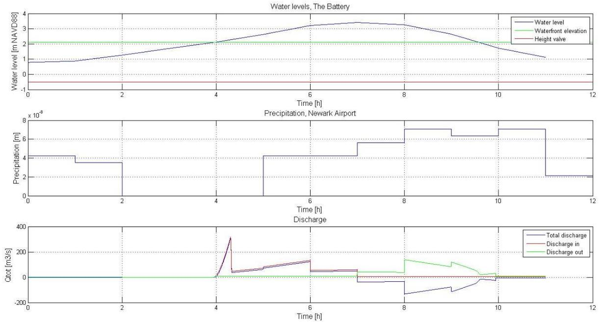
**Figure 24 Model results during overflow (Hurricane Sandy Hoboken): Water levels (plot 1); Precipitation (plot 2); Inflow and outflow fluxes (plot 3)**
