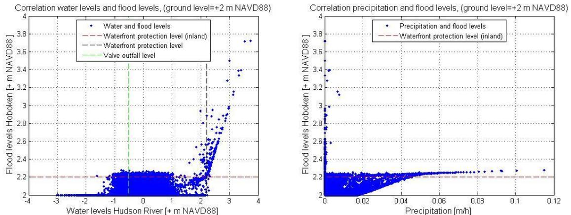
**Figure 41 Left: correlation water levels and flood levels; right: correlation precipitation and flood levels 1,000 years**
