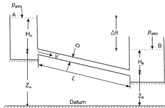
Figure 22 Flow of water from reservoir A to B (NPTEL)
