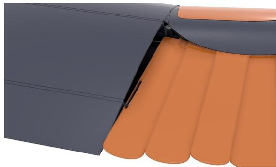
Figure 6.28: View of the inner platelet pin-channel connection to the trailing edge spar
