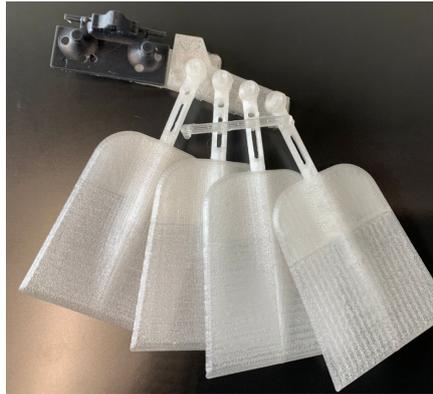
**Figure 13.3:** Picture of the 3D printed tail mechanism of the Air-Guard drone
