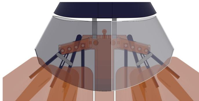
**Figure 5:** Detailed view of the tail morphing mechanism, in extended position
