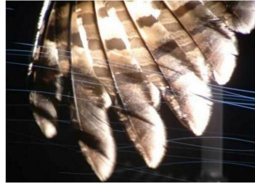
Figure 6.5: Wind tunnel effects of slotted wings [27]
