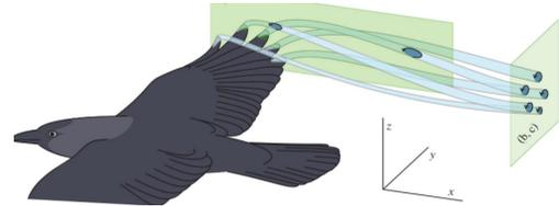
Figure 6.4: Effects of slotted wing tips on wing tip vortexes [27]
