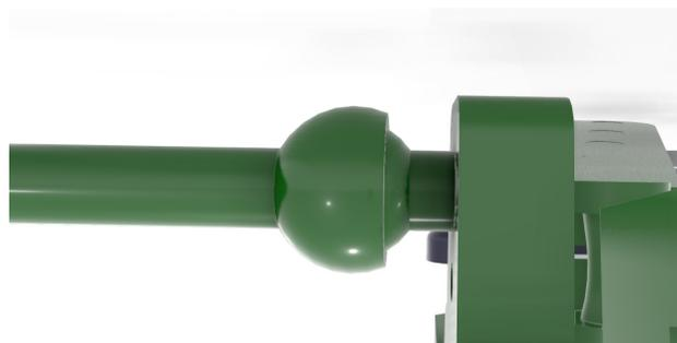
**Figure 7.15:** Ball and socket joint on the tail bracket for elevator deflection
