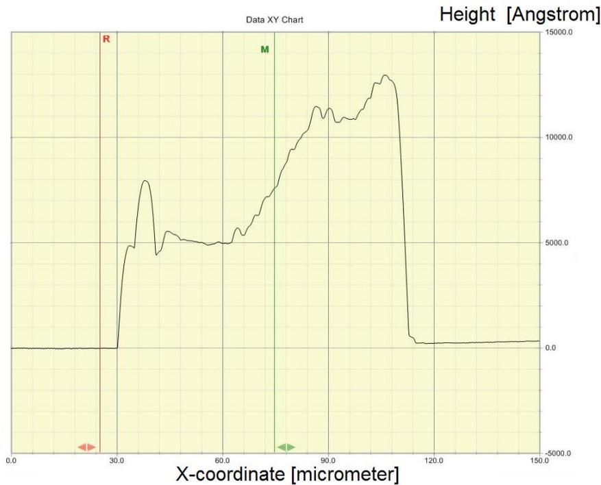
**Figure 29:** Height profile of nanocopper structure after NMP lift-off process.
