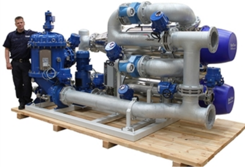
Figure 4.6: RayClean ballast water treatment system from Desmi [? ]
