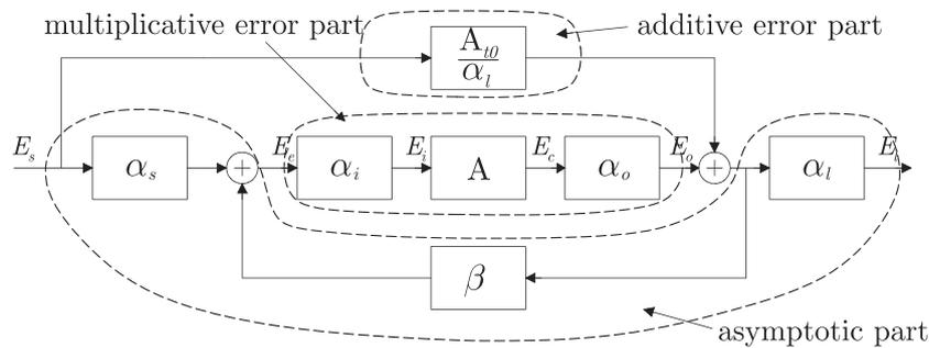
Figure 4. Single-loop synthesis model, hierarchically subdivided for synthesis: First, design the asymptotic part and then focus on the blocks in the error part.
