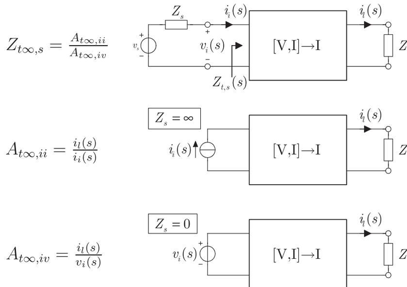
Figure 14. Input impedance of a feedback amplifier, calculated as the ratio between two transfers  $A_{t\infty,ii}(s) = i_l(s)/i_i(s)|_{A \rightarrow \infty}$  and  $A_{t\infty,iv}(s) = i_l(s)/v_i(s)|_{A \rightarrow \infty}$ .
