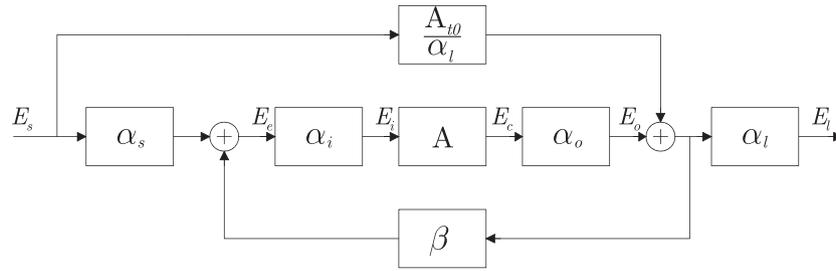
Figure 3. The complete single-loop synthesis model explicitly including all essential blocks for the evolution towards the double-loop feedback model.
