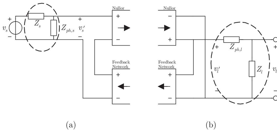
Figure 7. Attenuations *outside* the feedback loop at the source (a) and load (b), due to, for example, the implementation of a phantom-zero (frequency compensation) at the input ( $Z_{ph,s}$ ) and output ( $Z_{ph,l}$ ).
