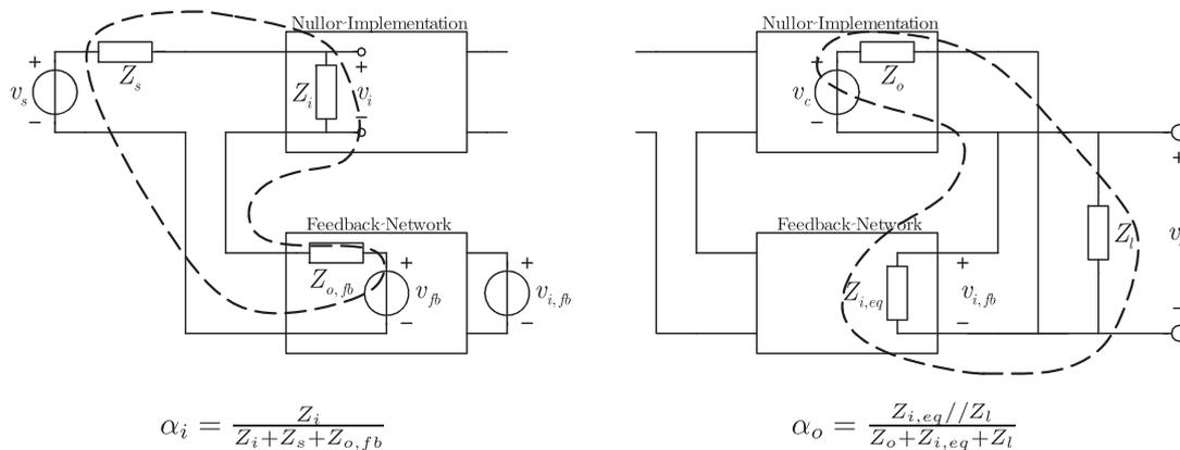
Figure 8. Attenuations *inside* the feedback loop at the input (left) and output (right) of the active part, due to a non-ideal input ( $Z_i$ ), respectively, output impedance ( $Z_o$ ) of the nullor implementation.  $Z_s$  is the source impedance,  $Z_l$  the load impedance.
