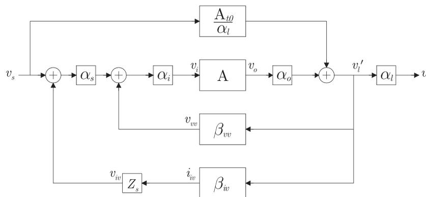
Figure 15. Synthesis model of a  $[V,I]$ -to-voltage amplifier with the voltage-to-voltage feedback network in the inner feedback path.
