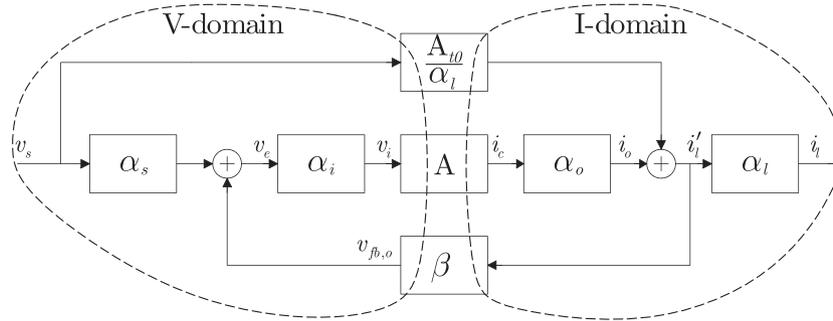
Figure 5. Single-loop synthesis model showing the assignment of the electrical signal quantities: A voltage and current have been assigned to the input and output branches of the model, respectively, for the example of a voltage-to-current amplifier.
