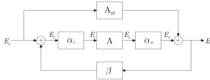
Figure 2. Synthesis-oriented single-loop feedback model, including input and output attenuations  $\alpha_i$  and  $\alpha_o$ , respectively, and direct transfer  $A_{t0}$ .
