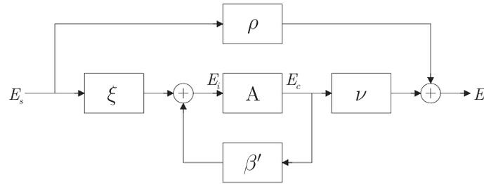
Figure 1. The asymptotic-gain model, which is not optimally suitable for the purpose of full synthesis.
