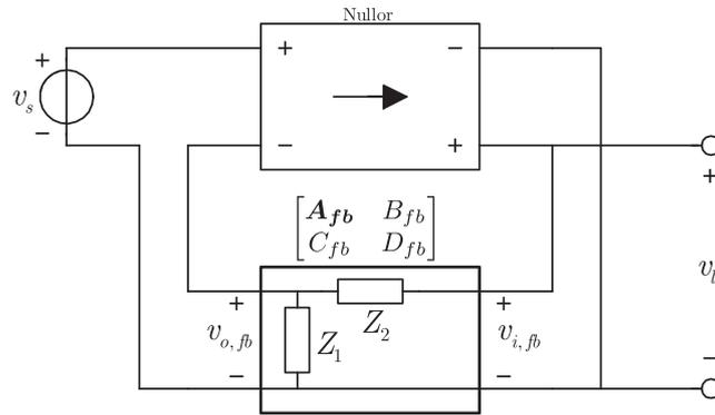
Figure 6. Interpretation of feedback block  $\beta$  in case of a voltage feedback amplifier.
