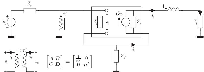
Figure 9. Double-loop feedback [V,I]-to-current amplifier. The ideal transformer, used here as current attenuator in the outer feedback network, and its chain matrix are shown in the corner.
