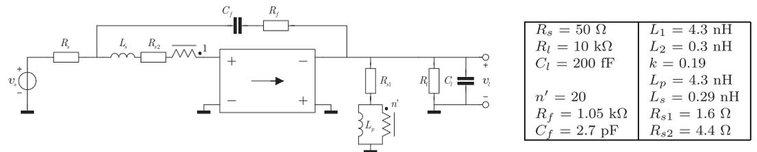
Figure 17. Schematic diagram of the transformer feedback [V,I]-to-voltage amplifier that fully defines its asymptotic behavior.
