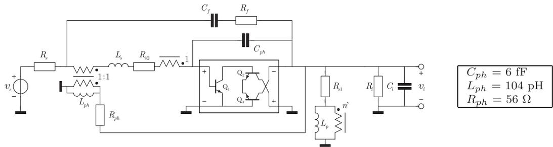
Figure 20. Schematic diagram of the complete transformer feedback [V,I]-to-voltage amplifier including the phantom-zero implementation corresponding to trace (IV) of Figure 19. In practice, the phantom-zero transformer can be combined with the main feedback transformer without any area penalty.
