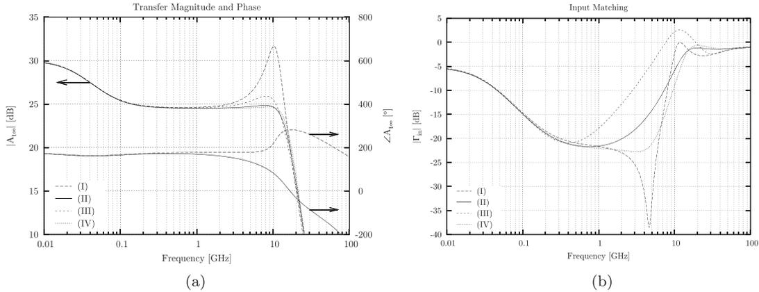
Figure 19. Simulated small-signal behavior: transfer magnitude and phase (a) and input matching (b). Legend: (I) no frequency compensation, (II) phantom zero in both feedback networks, (III) phantom zero in outer network only, and (IV) phantom zero in both feedback networks, but skewed to compensate for the high-frequency roll-off of the loop gain.
