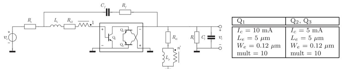
Figure 18. Schematic diagram of the transformer feedback [V,I]-to-voltage amplifier with the small-signal implementation of the active part.
