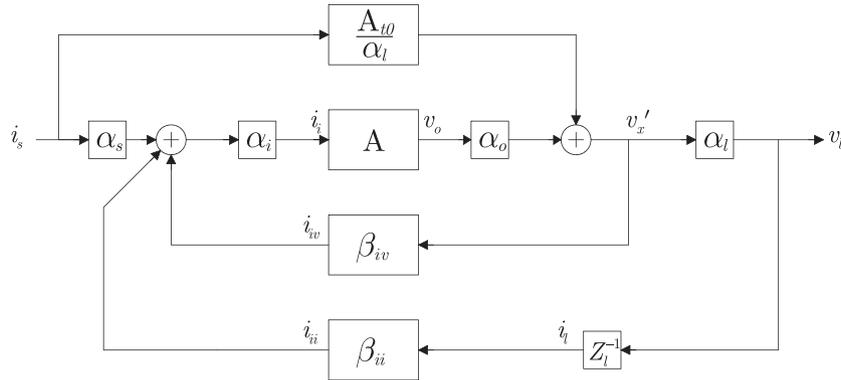
Figure 13. Double-loop synthesis model of a current-to-[V,I] amplifier with current attenuation feedback network in the output loop.
