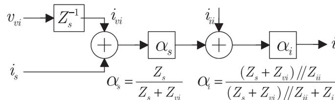
Figure 12. Norton transformation of feedback voltage  $v_{vi}$  and the appearance of source attenuation  $\alpha_s$  due to the current division from  $Z_s$  and the non-zero output impedance  $Z_{vi}$  of the  $i \rightarrow v$  feedback network.
