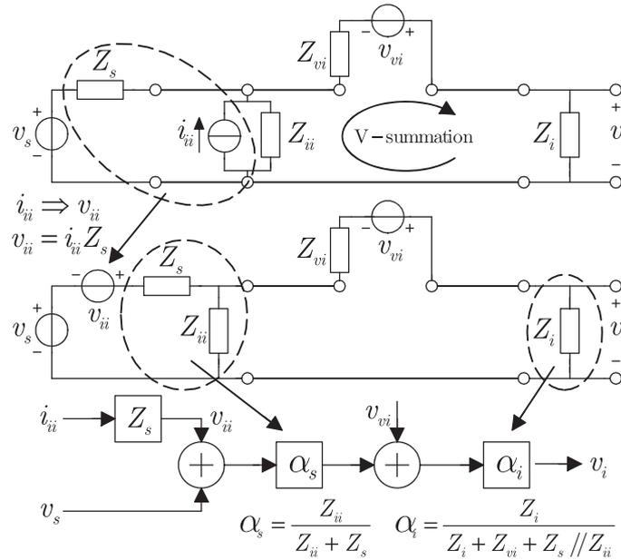
Figure 11. Thévenin equivalent of the feedback current  $i_{ii}$  and the appearance of the source attenuation  $\alpha_s$  due to a finite output impedance  $Z_{vi}$  of the current feedback network.
