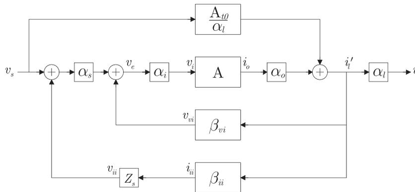
Figure 10. Double-loop synthesis model of a [V,I]-to-current amplifier.
