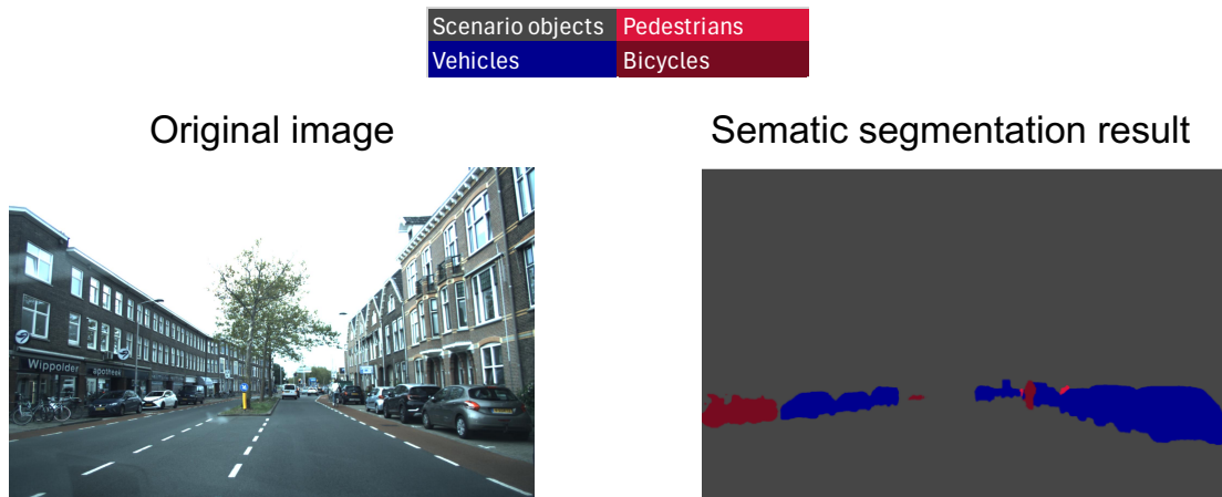
Figure 4.4: The original optical image and the corresponding semantic segmentation result for the same complex scenario shown in Figure 4.1. As it can be observed, nearly every pixel is correctly segmented
