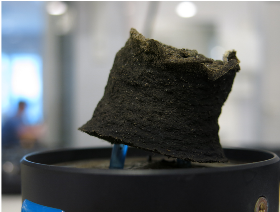
Figure 6.1: Bend of the top tensiometer due to the shrinking soil - Non-oxidised & partially air dried Hyprop campaign
