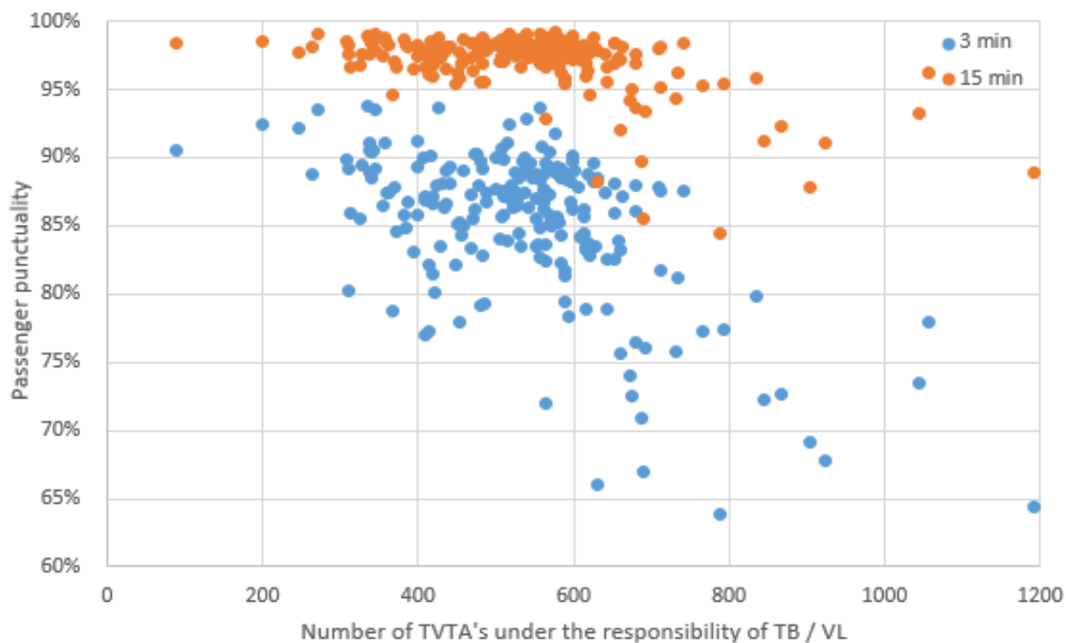
Figure 5.4: The number of TVTAs versus the passenger punctuality for 181 days for the business unit TB / VL
