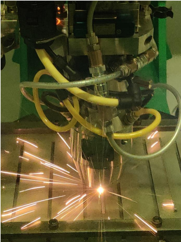
Figure 47. AM of a layer of pure SS316L in the bimetal structure. (b) AM of a layer of pure In718 in the pure In718 structure. Note the considerable less sparks in the In718 build, as it experiences less oxidation.
