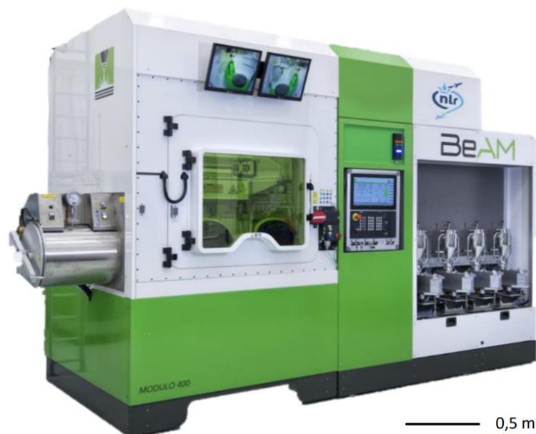
Figure 15. BeAM Modulo 400 as part of the research facility of NLR. Note the four powder hoppers at the right side of the machine.
