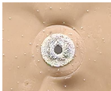
Figure 35. Results of post-experimental laser alignment test. Showing the hole created by the laser in the middle of the circle area of powder particles.
