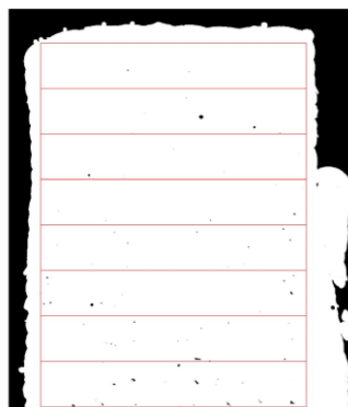
Figure 41. Structure 1, type 10 wt% FGM, the red outlined regions represent the 8 sections in which the porosities have been determined.
