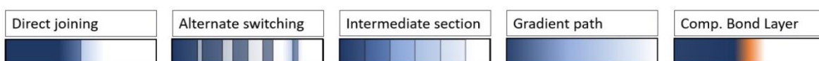
Figure 6. Build methods to produce an FGM transitioning the composition from one metal to another [16].
