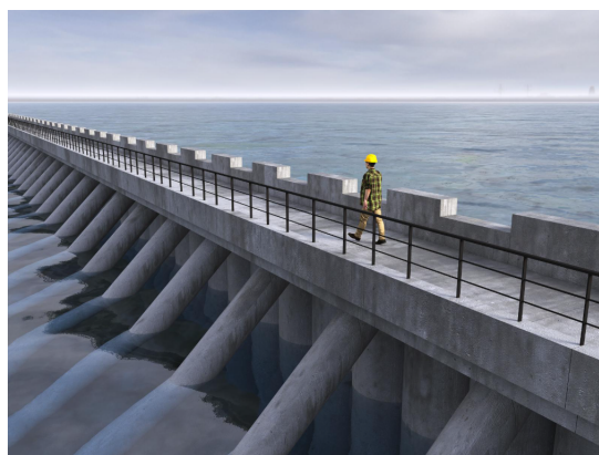
(a) Conceptual rendering of the combi-wall section (USACE, 2021d).
