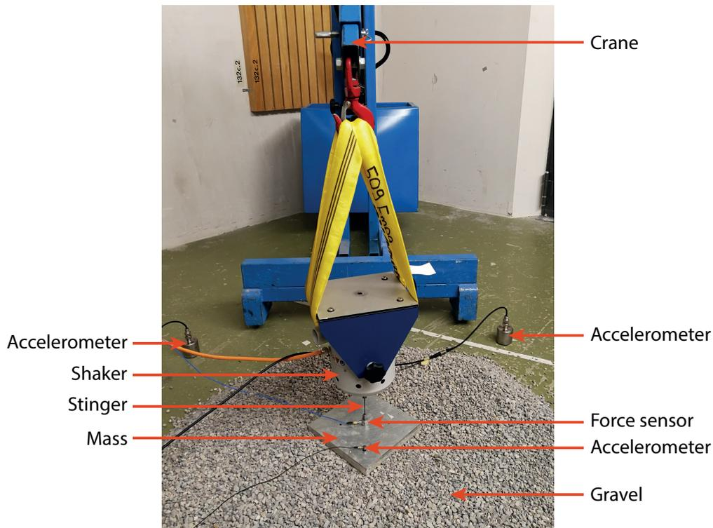
Figure 5-1: Apparatus for transmission tests.
