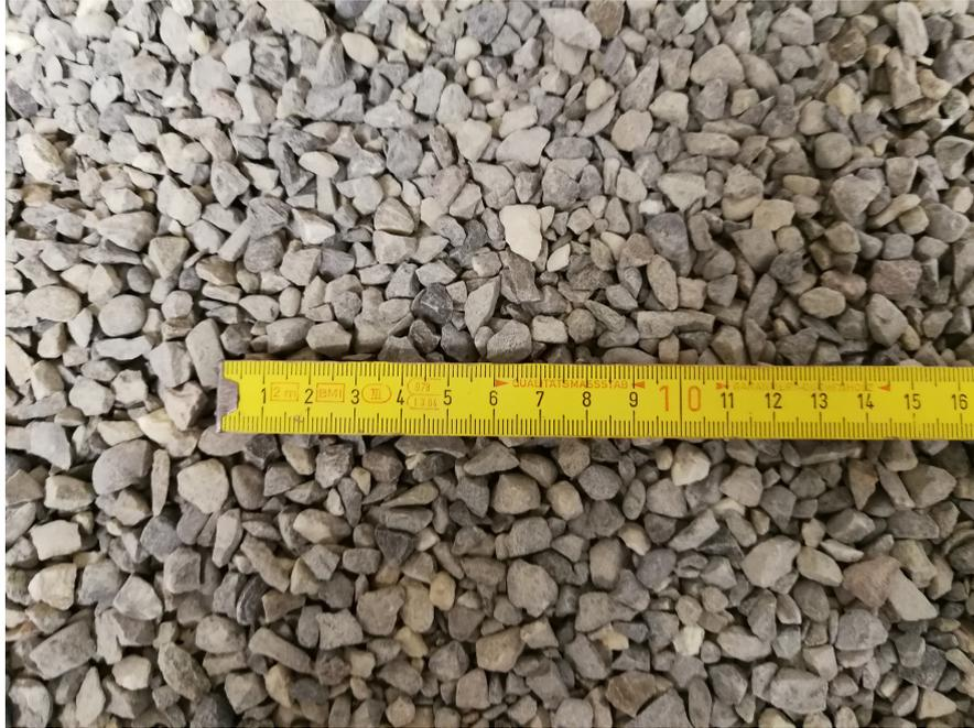
**Figure 3-1:** Small-scale railway ballast, *gravel*.
