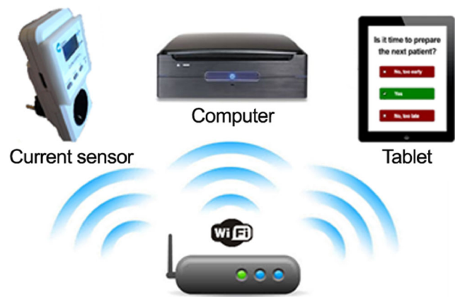
Fig. 2 Schematic overview of the real-time prediction system
