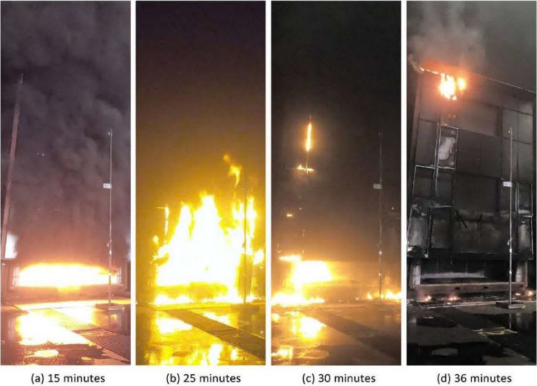
Figure 2: Large scale test BIPV facade. Impact falling BIPV modules. Source: Stølen et al. (2024)
