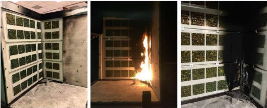
Figure 1: SBI-test with PIZ BIPV cladding system. Source: IEA PVPS Task 15 (2023)
