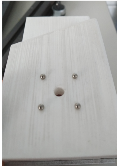
(b) A connection between the 3D printed components, showing the bolthole and steel balls for centring.
