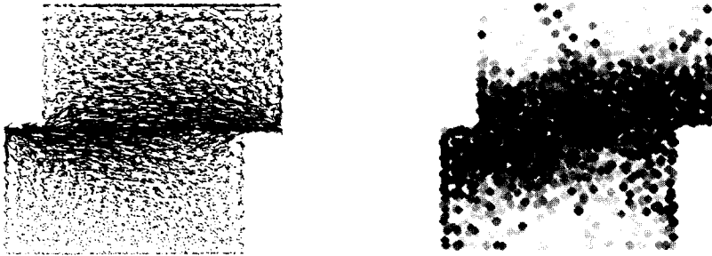
Figure 6.10: Trajectories (left) and rotation around the z axis (right) of the particles projected on the xy plane. The shear deformation is 32 \mu\text{m} . The rotation of a particle is given by a dot; the larger the rotation, the darker the dot.
