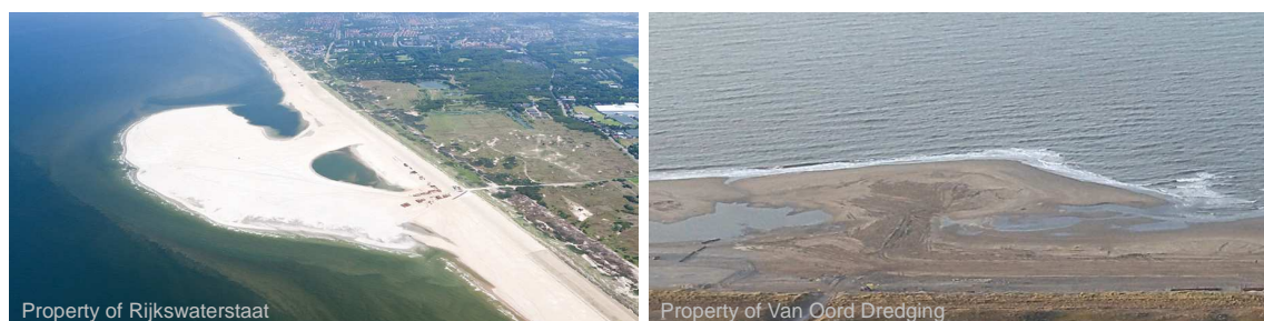
Figure 1. Examples of nourishments along the Dutch coast. Left : ‘Sand Motor’ between Monster and Kijkduin in July 2012 ; Right : ‘Sand groynes’ at Monster in October 2009 (Hoekstra et al., 2012)
