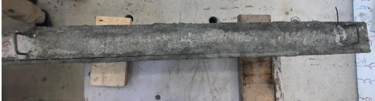
**Figure 3.12:** Delamination in the beam which is clearly visible.
