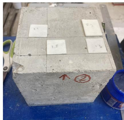
(b) Simulating the delaminated areas of the second sample with PIR.
