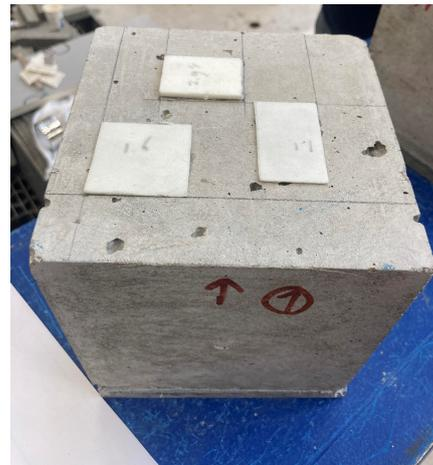
(b) Simulating the delaminated areas of the first sample with PIR.
