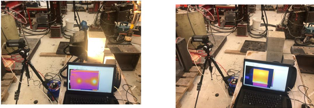
(a) Setup of heating the specimen with close-by heating with a halogen lamp. (b) Setup of recording the cooling the specimen.
