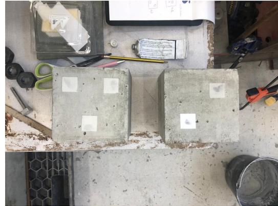
(b) Test sample with three delaminations at a bigger distance from each other and a test sample with two delaminated areas with thicknesses of 0.1mm made of paper and 0.5mm made of PIR.
