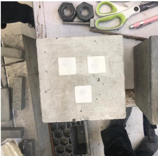
(a) Test sample with three delaminations at small distance from each other.
