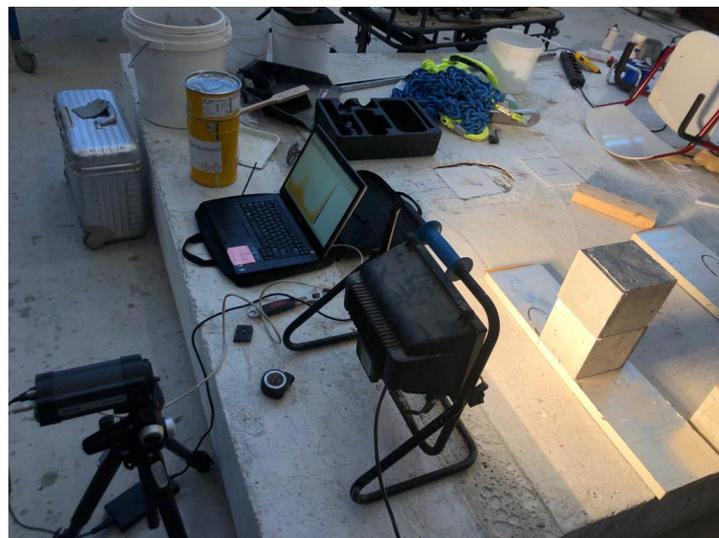
**Figure 3.9:** Heating the test sample from 40cm distance with a halogen lamp.
