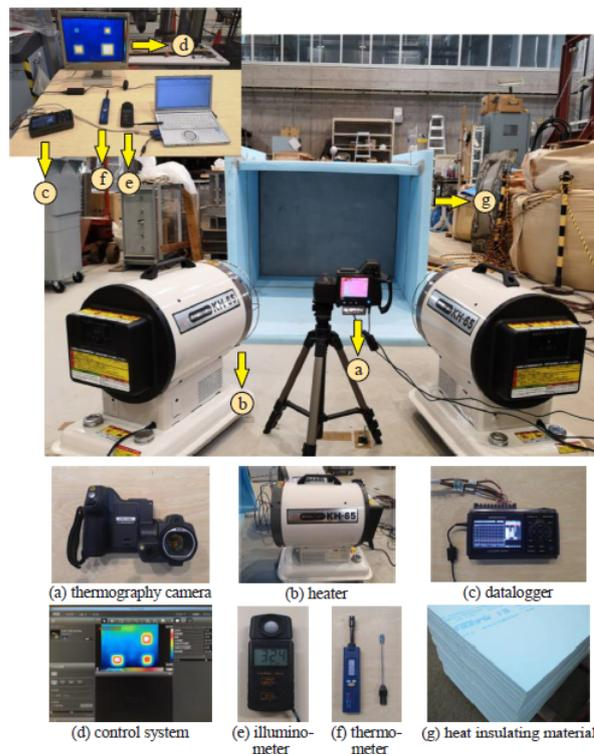
Fig. 4. Setup of the experiment.
