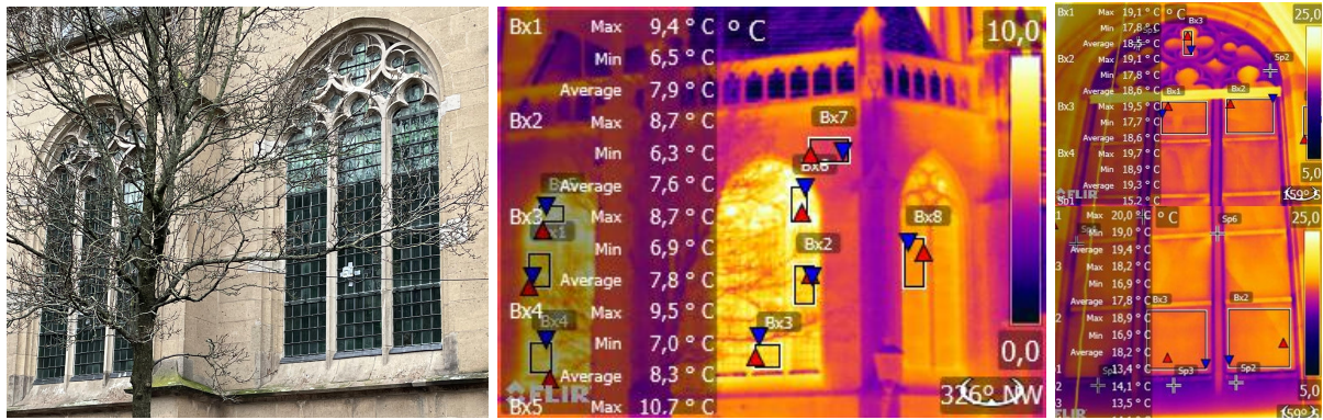
Figure 3.9: Windows with internal PG Gerfkamer - Photograph (l) and thermal image outside (c) and inside (r)
