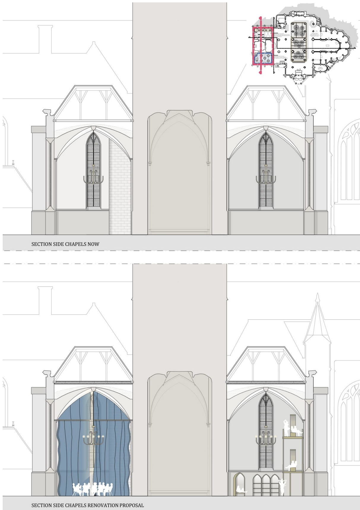
Figure B.8: Section Stevenskerk - South chapel with textile radiation screen, North chapel with walkways
