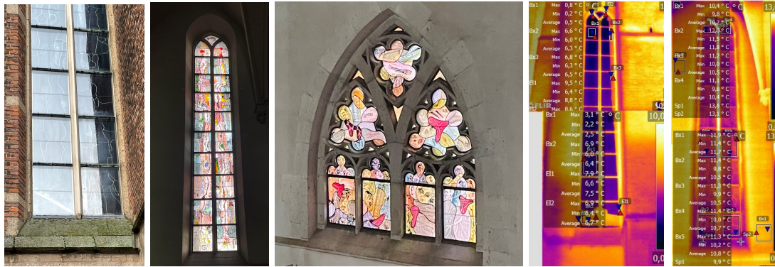
Figure 3.10: Painted glass windows with external PG - Photographs (l) and thermal images (r)
