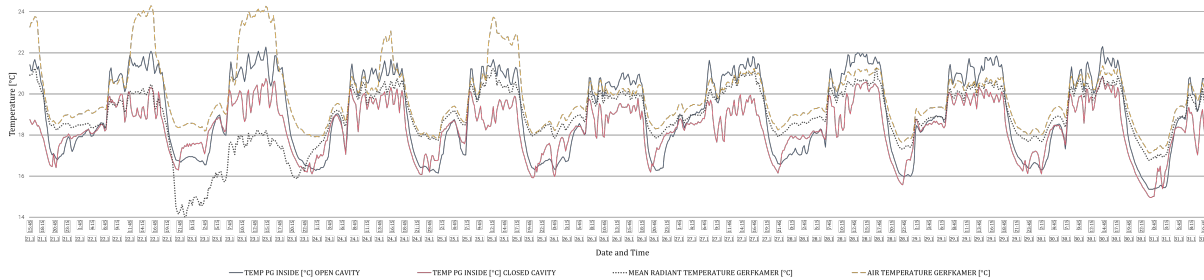
Figure 5.6: Graph full measurement period Gerfkamer: Internal surface temperature window open and closed cavity, air temperature and MRT
