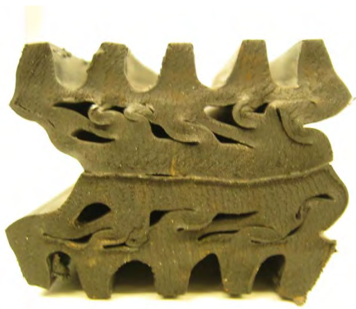
figure 4: Permanent deformation of the gasket after heating
