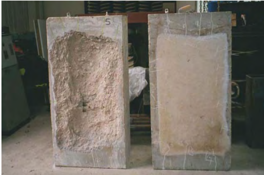
FIGURE 19: FIRE TESTED CONCRETE SLABS WITHOUT (LEFT) AND WITH (RIGHT) PP-FIBRES [39]
