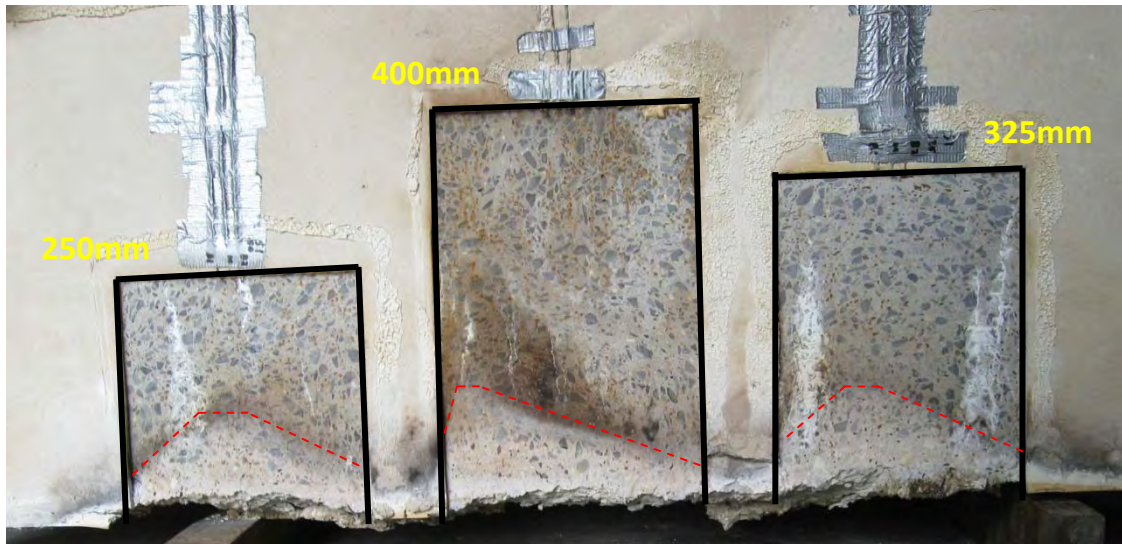
figure 14: Flame intrusion paths in the gaps of sample 2
