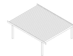
20m Grid: 20m span, 1200mm deep
