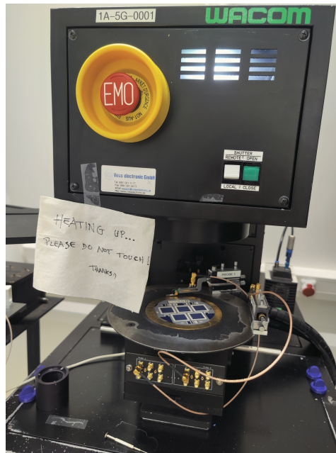
Figure 3.4: The WACOM Solar Simulator measurement set-up with the gold-plate NIP stage for variable temperature measurements, underneath the cells' wafer.
