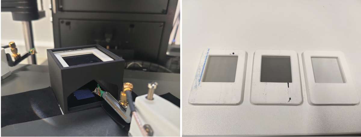
Figure 3.5: The irradiance measurement set-up, featuring: (on the left) a 3-D printed holder for the irradiance filters, custom-made to fit over the c-Si cell. (on the right) the irradiance filters utilised to scale down the intensity hitting the cell, mounted inside 3-D printed white covers for proper handling (note the different luminosity of the glasses, according to the filter's transmittance capability).
