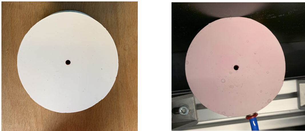
(a) Compliant bearing before being used with the solution of water and Rhodamine B. (b) Pink coloured bearing surface as a result of the Rhodamine B particles sticking
