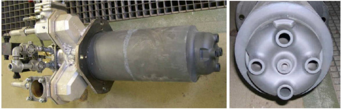
Figure 2.7: REGEMAT® CD 200 regenerative burner used in the multiburner flameless furnace of TU Delft (from [36])
