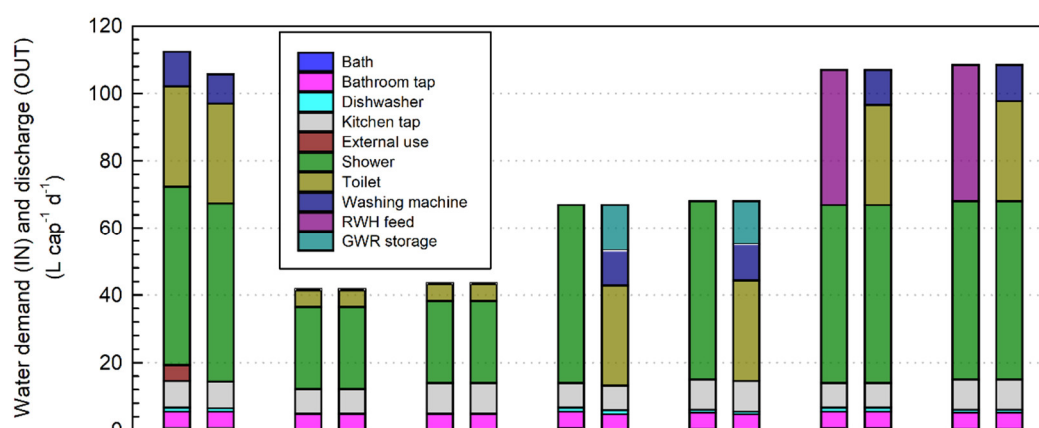
Figure 2. Outline of appliance demand and discharge for each of the future scenarios.
