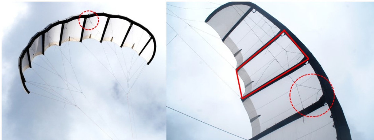
Figure 3.2: Two images of the V3 kite. The red quadrilateral indicates one of the spanwise segments, and the red circles indicate the bridle fan [1].
