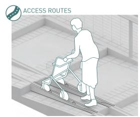
[1] tracks enable the use of wheeled devices on stairs with backstoppers that give traction to minimize the effort of pushing device
