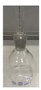
Figure 9 - Water displacement pycnometer
