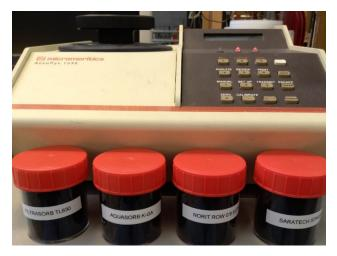
Figure 8 – Accupyc pycnometer.
