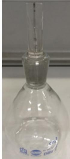
Figure 9 - Water displacement pycnometer
