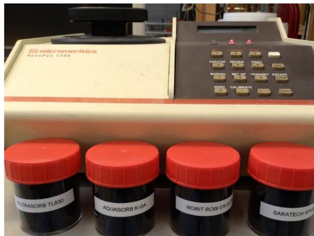
Figure 8 – AccuPyc pycnometer.
