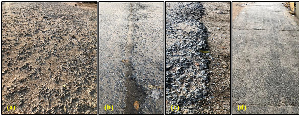
Figure 3. Structural defects: (a) severely ravelled pervious concrete pavement slab, (b) joint deterioration, (c) edge cracking and (d) skid marks.
