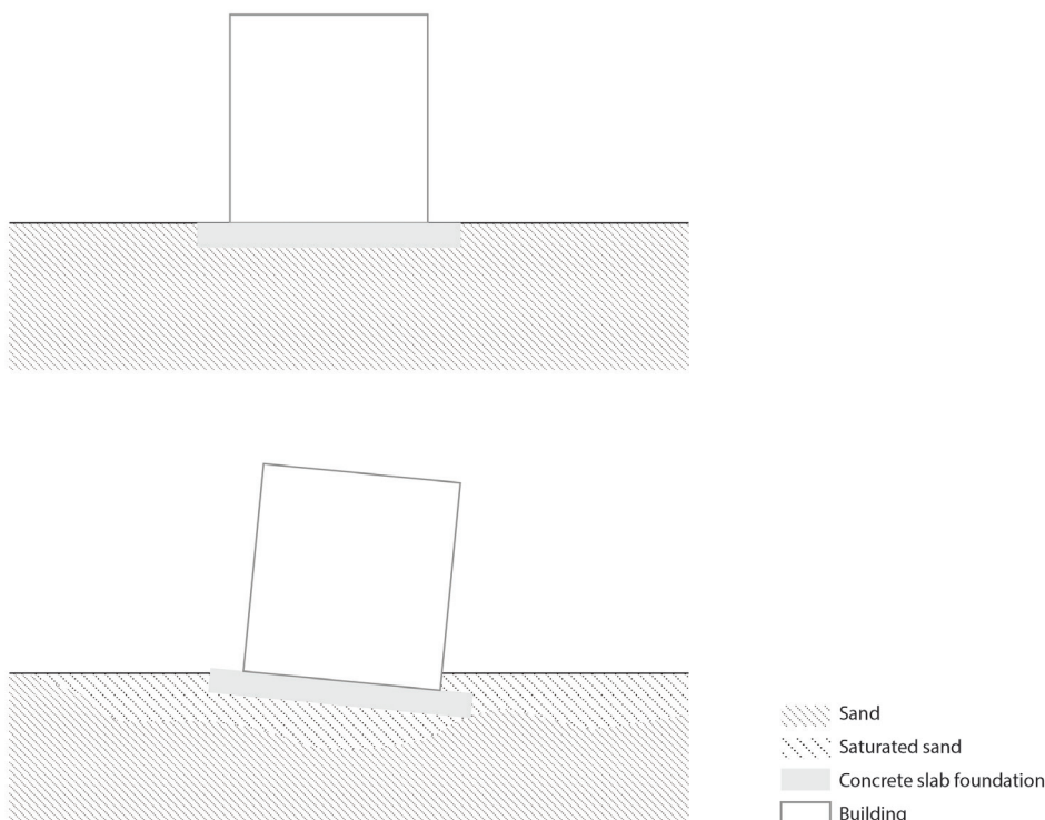
▲ figure 50. The effect of liquefaction on a building with concrete slab foundation. Author
