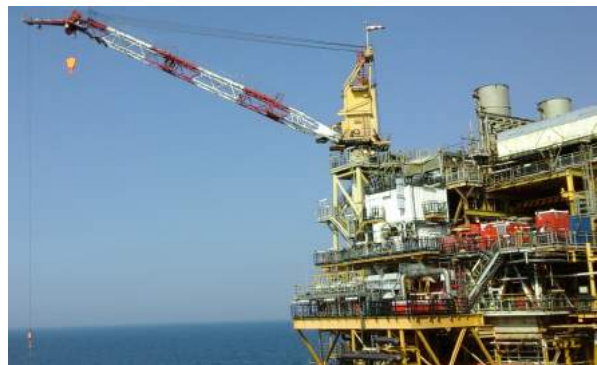
Figure 3.5: A permanent mounted platform crane
